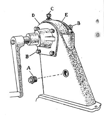
At the rear of the gear housing is placed a grease cup. Use this grease cup regularly but never much at a time. The grease from this cup lubricates the sealing rings. Without grease these rings can be damaged.
